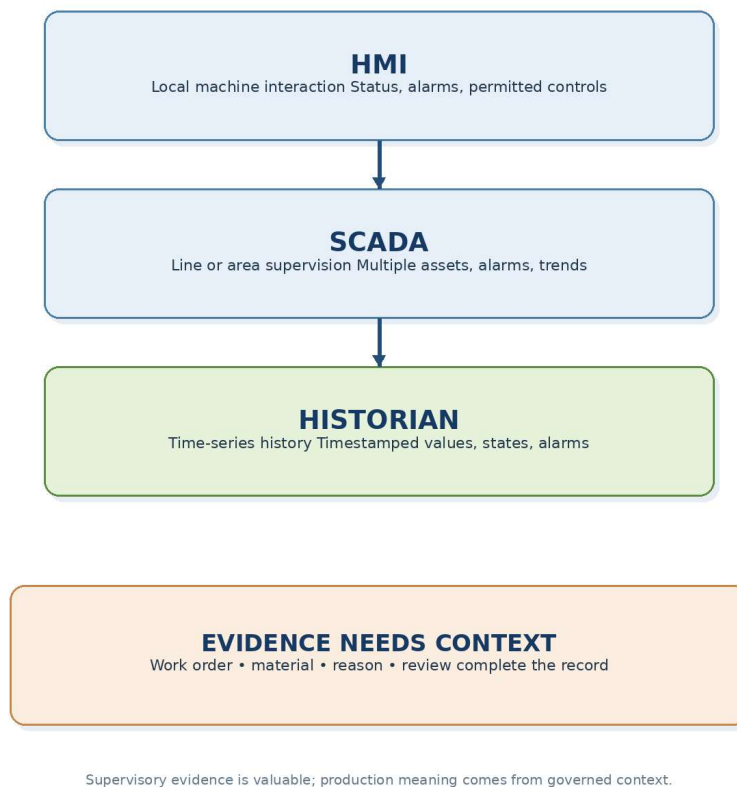
Figure 4.1: HMI, SCADA, and historian.
